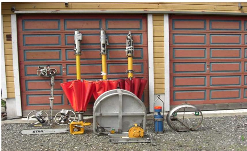
Fig. 4 Tools for sediment sampling and sea ice drilling developed for the hovercraft.
